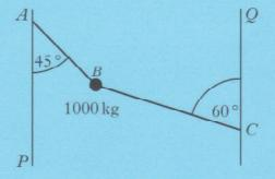
PA and CQ are vertical with  $\angle PAB = 45^{\circ}$  and  $\angle BCQ = 60^{\circ}$ . The tensions in the chains over sections AB and BC are denoted by  $T_1$  and  $T_2$  respectively.
