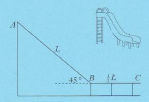
Starting from rest, Jill slides down the chute from A to C. Over both sections of the chute a frictional force acts on Jill where the coefficient of friction between her and the chute is  $\frac{1}{2}$ .
