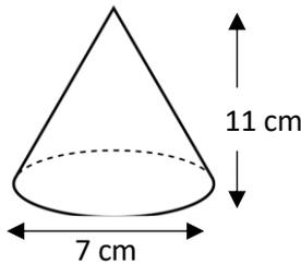
$$\begin{aligned} \text{Volume} &= \frac{1}{3} \times \pi \times (3.5)^2 \times 11 \\ &= 141.10987\dots \\ &= 141 \text{ cm}^3 \end{aligned}$$
