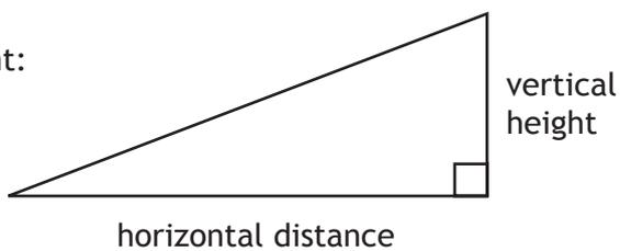
$$\text{gradient} = \frac{\text{vertical height}}{\text{horizontal distance}}$$
