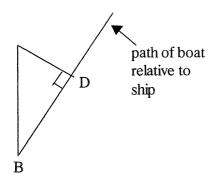
Path of boat is in the direction of  $v_B - v_S$ .
