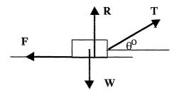
As the block is on the point of moving  $F = \mu R$ Resolving vertically:  $R + T\sin\theta = W = mg$ Resolving horizontally:  $T\cos\theta = F$
