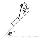
If the coefficient of friction is  $\frac{1}{\sqrt{2}}$ , calculate the magnitude of **P** if the particle is on the point of moving up the plane.
